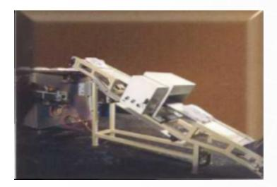
The Detec Series 4B range of metal Detectors is designed and proven to meet food and pharmaceutical health and safety standards.
